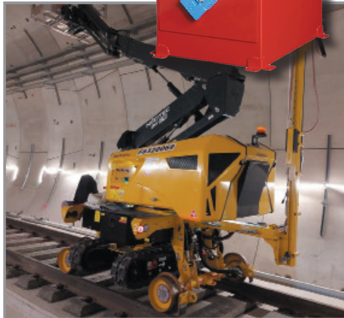
LEFT: The Flash Battery 51.2V-200Ah-10kWh lithium battery solution
