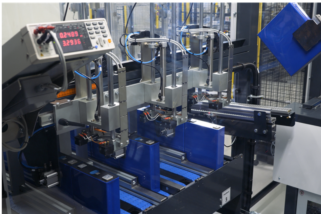
Individual battery cells are loaded into modules - these are later combined into packs
