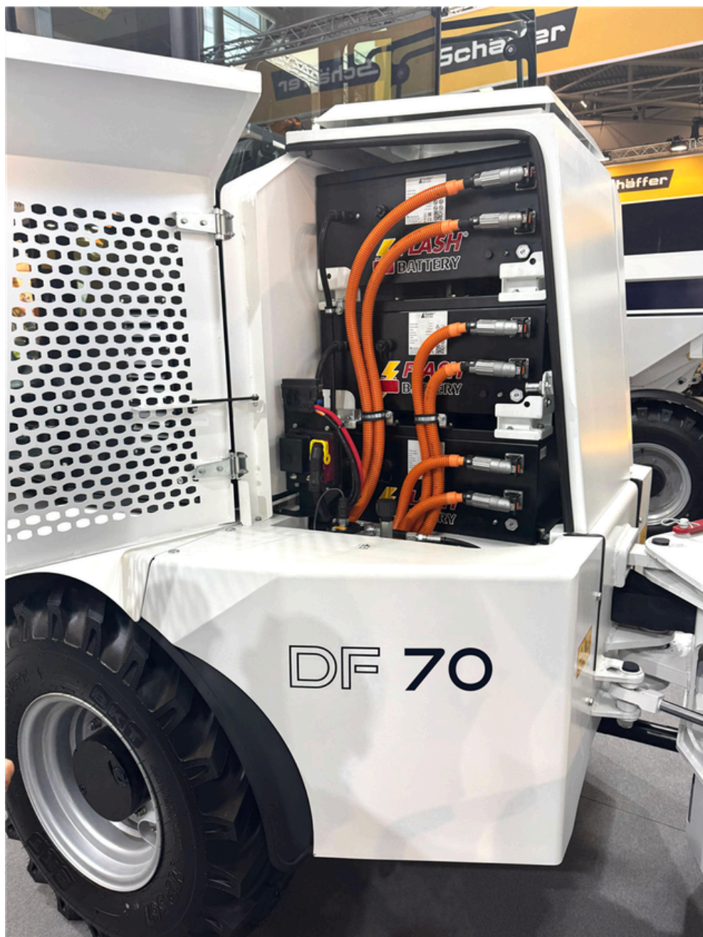
Fiori has worked with Italian battery manufacturer Flash Battery on electric versions of its site dumpers, Image: Fiori
